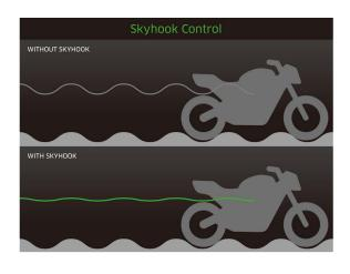
both the suppleness to offer riding comfort in a wide range of riding situations, as well as the firm damping to facilitate sport riding. The tyres feel planted, delivering confidence when cornering. In Rain Mode, Showa's Skyhook EERA (Electronically Equipped Ride Adjustment) technology offers an even more composed ride.
