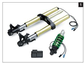
\* Base damping character is set according to the integrated Riding Mode (Sport, Road, Rain, Rider (manual)) selected. KECS then adjusts to the road surface environment in real time to provide the ideal damping, taking into account vehicle speed, stroke speed and deceleration.
